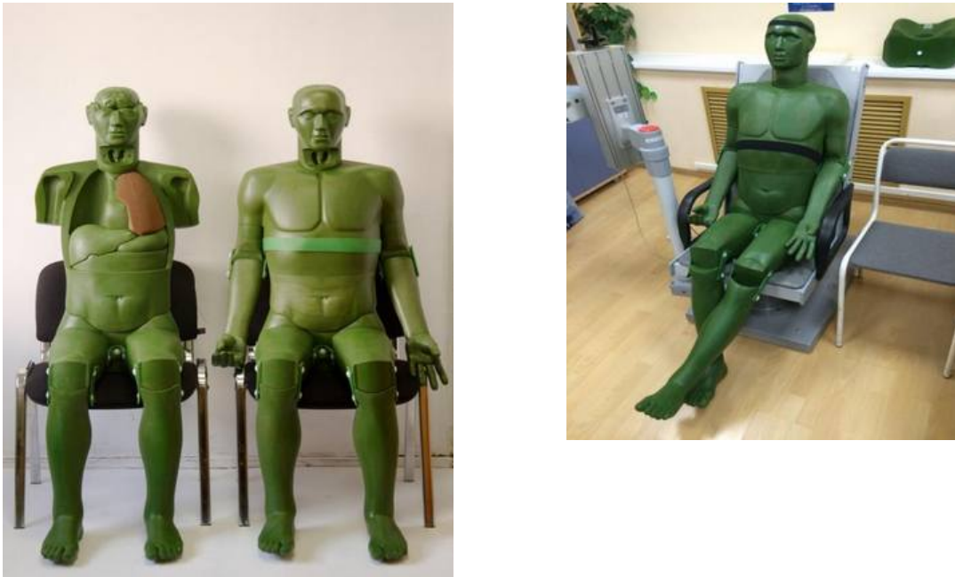
Figure 1 – Phantom of the human body and organs in the measuring position in a whole body counter at NPP, measurement of ^{60}\text{Co} in the lungs
